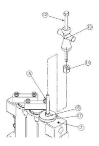
Note: FMC M12 valves are held in place using a self-locking taper. The tapered portion of the valve seat and the tapered portion of the fluid cylinder must be clean and dry prior to assembly to insure proper operation. Failure to properly clean parts before reassembly could lead to wash out of fluid cylinder or dislodgment of valve assemblies during operation.
